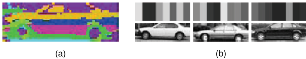
Figure 2.13: The Probabilistic Index Map method (Jojic and Caspi, 2004). Given a set of input images (bottom), the model learns a distribution on index maps (a sample from which can be seen on the left) that captures the colour-invariant structure in the data. Latent ‘palettes’ (top) are inferred to explain the data. Labelled training data can be used in conjunction with the index maps to perform object segmentation.
