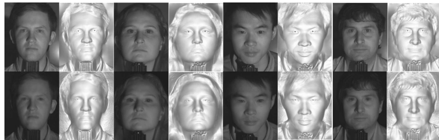
Figure 3: Example raw images and reconstructions using visible (top) and NIR light sources for four subjects. For these experiments only, the subjects were asked to rest their chin on a support in order to ensure that all subjects are compared to each other in fair conditions.
