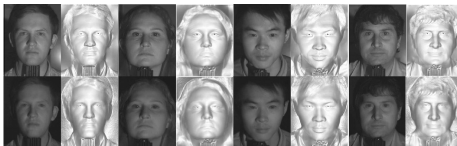
Fig. 4. Example raw images and reconstructions using visible (top) and NIR light sources for four subjects. For these experiments only, the subjects were asked to rest their chin on a support in order to ensure that all subjects are compared to each other in fair conditions.
