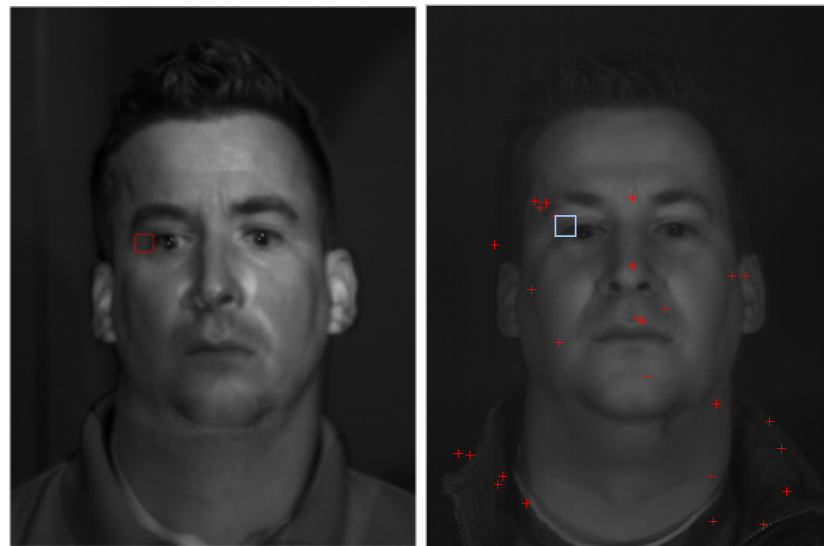
Figure 8.3: Landmark feature detection using Haar-like features from the method of Viola and Jones. Highest scores for the albedo image (left) and y -component (right) using the 100 top performing features. The top score for the albedo is located very close to the actual left lateral canthus (red square), but there are many false hits for the surface normal data (the blue square indicates the closest match).
