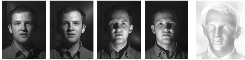
Figure 2: Example of four raw images and the resultant surface reconstruction.
