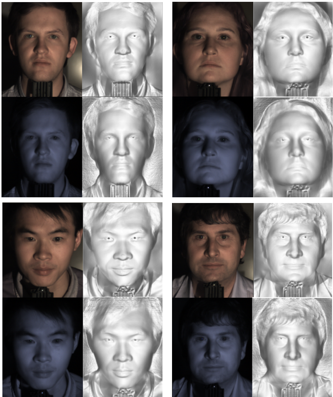
Figure 3.4: Example raw images and reconstructions using visible (top) and NIR light sources for four subjects. For these experiments only, the subjects were asked to rest their chin on a support in order to ensure that all subjects are compared to each other in fair conditions. Note that hair is well recovered (other methods e.g. 3dMD tend to reconstruct hair poorly).
