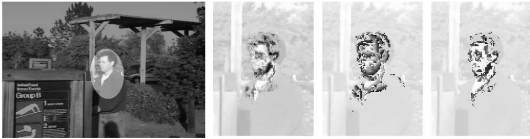
Figure 2.3: The WSL tracker [Jepson 03] estimates components on a template that are reliable for tracking. This increases the tracker’s robustness to partial occlusion and appearance changes.
