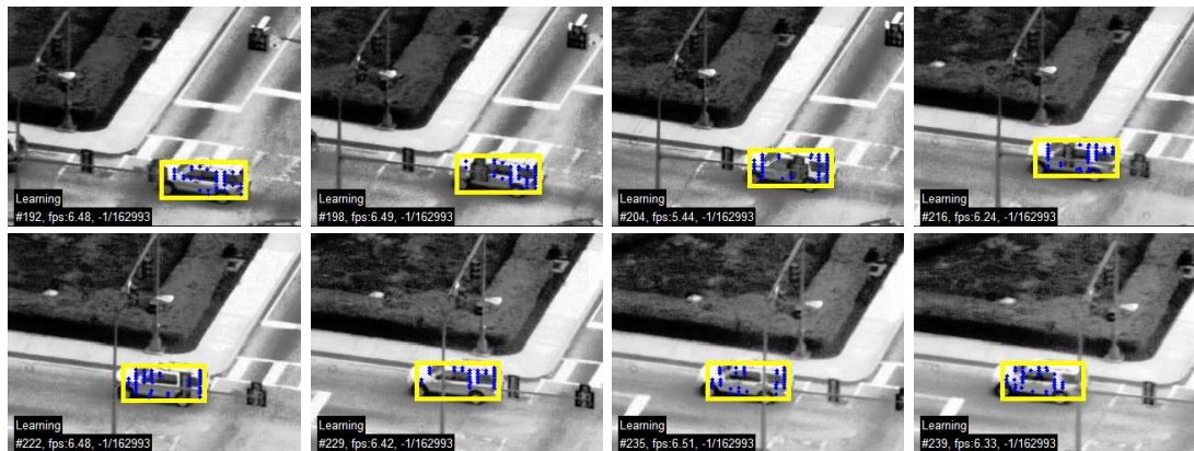
Figure 3.7: Several frames from the sequence CAR overlaid with the output of the Median-Flow tracker (yellow) and 50% of the most reliable points (blue). Notice that the points are covering the visible parts of the tracked object. The points that cover occluded or low-textured parts of the object are automatically filtered out by the Forward-Backward error.
