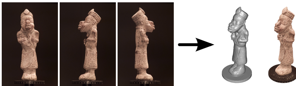
Figure 1.5: Example of current state-of-the-art reconstruction. The images of the statue have been taken on a turntable against a fixed background and reconstructed using [Hernández and Schmitt 2004].
