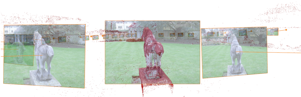
(b) Example of the recovered camera calibration and triangulated 3D 'point cloud'
