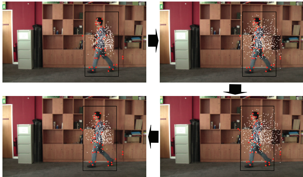
Figure 3.28: The propagation of particles. The top row shows the same frame but with the initial set of particles (left) and the set of particles after they have been allowed to perform a random walk (right) before being applied to the next frame. The bottom row shows the next consecutive frame, with the initial distribution (right) and the distribution after importance sampling (left). The resultant estimated position of the bounding box is also shown for each frame. The red circles show the set of foreground features being used and each white point shows the location of each particle that defines the centre of a bounding box.
