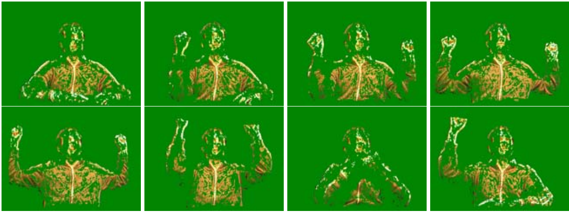
Figure 4.9: Examples of synthesised views using the original disparity maps from Figure 4.8. Camera 1 (see Figure 4.4(b)) is used as the virtual camera.
