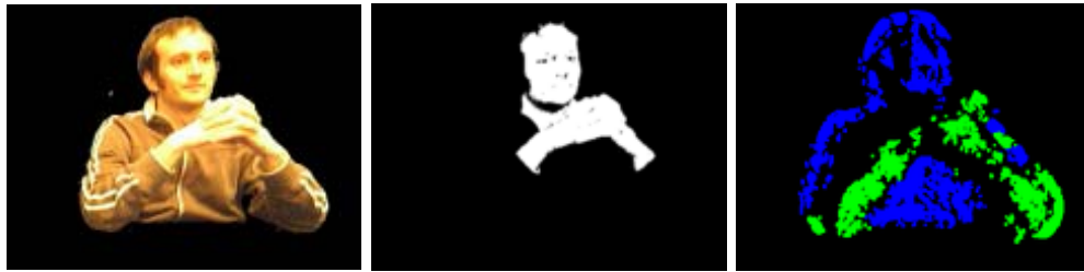
Figure 4.28: An example frame and its unsuccessful hand segmentation and disparity map segmentation.
