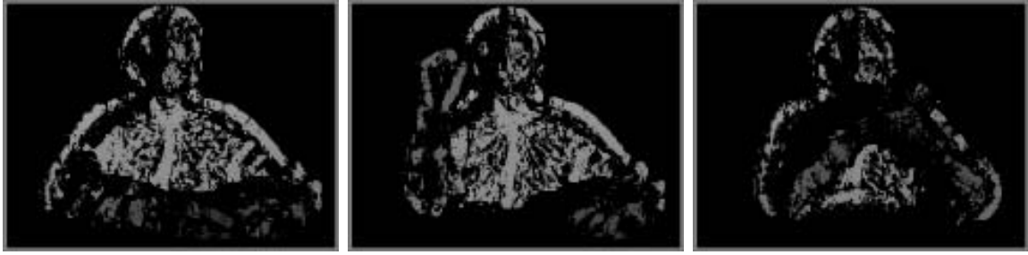
Figure 6.14: Examples of patchy disparity map data resulting from a correspondence search algorithm. The data shown in this figure passed the consistency check and the regions with no available disparity data are shown in black.
