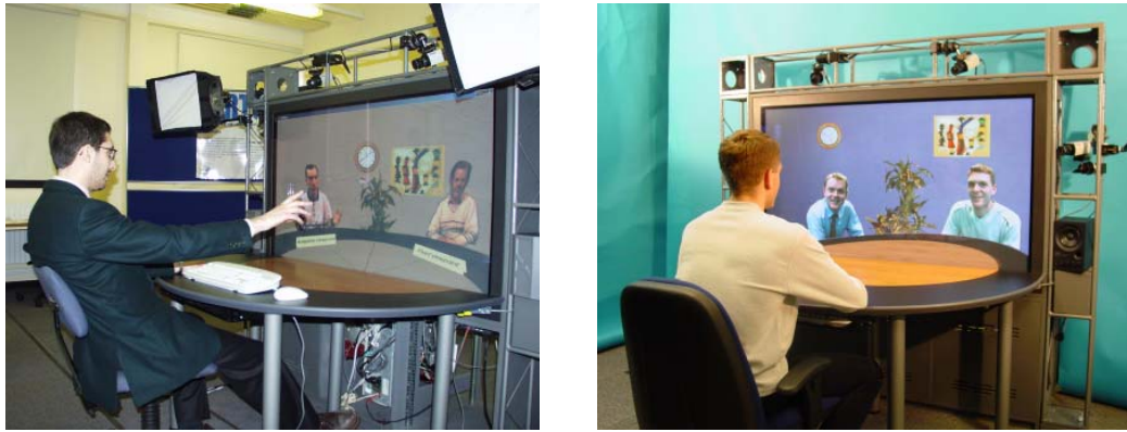
Figure 4.1: The VIRTUE videoconferencing station. 4 cameras were arranged around the screen in 2 wide-baseline stereo pairs.
