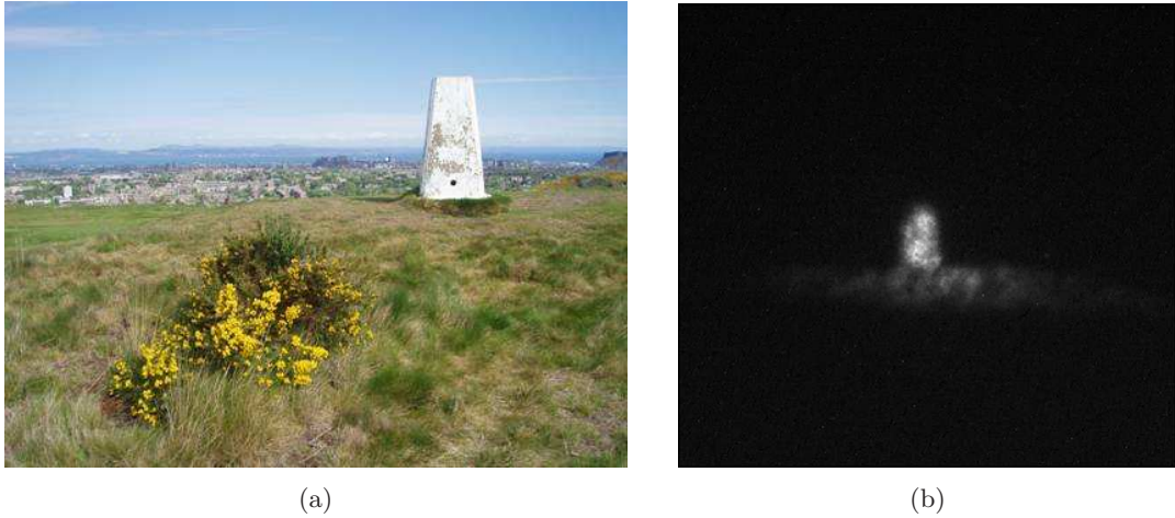
Figure 4.22: (a) UK Ordnance Triangulation Point (trig point) (b) Single frame BIL image of a trig point (long range)
