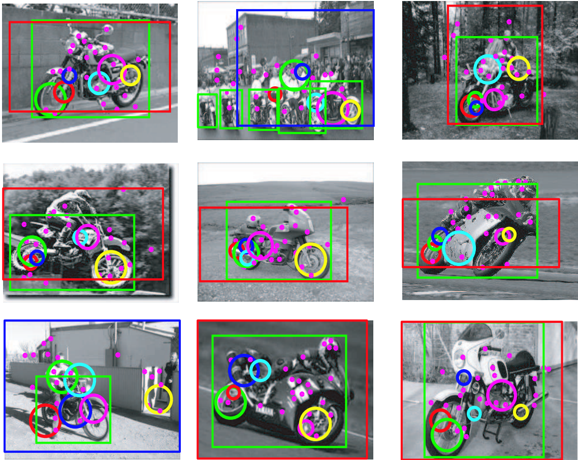
Figure 8.10: Examples of motorbikes from the PASCAL test set 2 being localized. The best hypothesis is indicated by the coloured circles and the background regions' centres' by the magenta dots. The ground truth bounding box is shown in green. A correct putative box is shown in red while an incorrect one is shown in blue.
