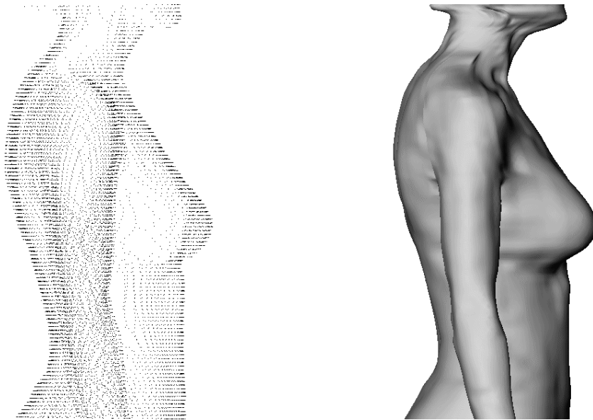
Figure 10: Examples of whole body surface reconstruction where interpolation has been used to cover gaps in the original data. The gaps occur at the side of the Torso. Left: Original point cloud (detail view of the torso, upper arm and neck segments), shown from a side view that illustrates the gaps in the sampling. Right: The same segment with a B-Spline surface fitted to it. Note the spurious features (ripples) arising at the gaps where there is insufficient data to drive the spline interpolation effectively.
