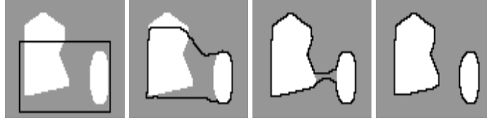
Figure 3. From left: the original image, initial CCM, and snapshots of contour propagation.
