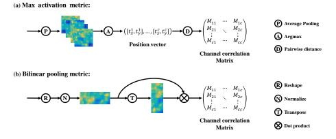
Figure 2: An illustration of channel correlation metrics: (a) max activation that groups channels into discriminative local region, and (b) bilinear pooling metric that groups channels based on visual pattern.
