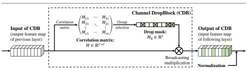
Figure 1: Illustration of the CDB block. The channel correlation matrix is generated based on different metrics. Then one channel and its corresponding visual group is randomly dropped by applying the drop mask to the input feature map.
