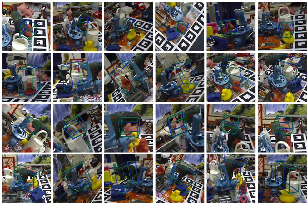
Figure 5: Visualization of qualitative results on the Occlusion LINEMOD dataset. Green 3D bounding-boxes represent the ground-truth poses and the blue ones indicate our predictions.
