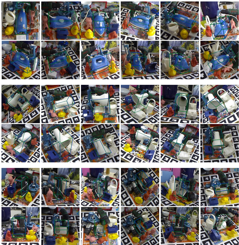
Figure 3: Visualization of qualitative results on the LINEMOD dataset. Green 3D bounding-boxes represent the ground-truth poses and the blue ones indicate our predictions.
