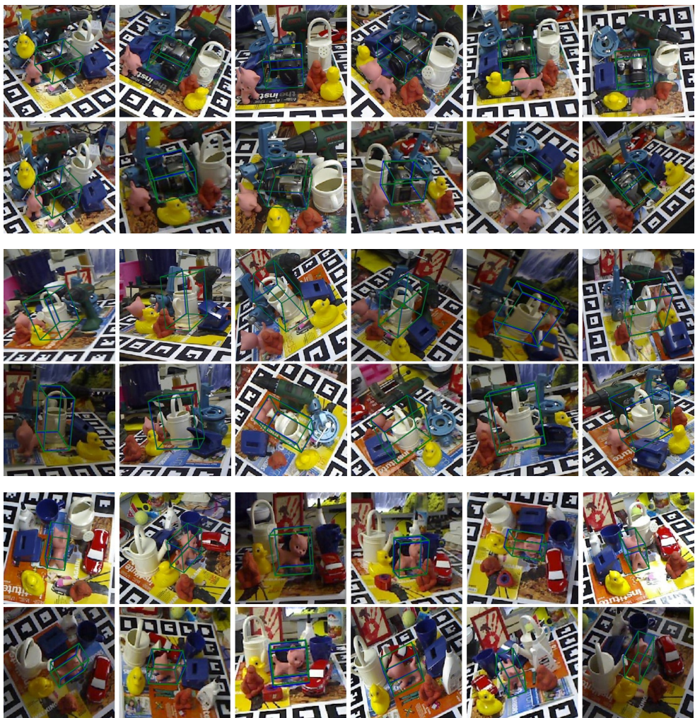
Figure 1: Visualization of qualitative results on the LINEMOD dataset. Green 3D bounding-boxes represent the ground-truth poses and the blue ones indicate our predictions.
