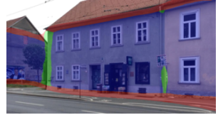
(c) Segmentation Result (blue: façade, green: vertical edge, red: horizontal edge).
