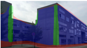
(c) Segmentation Result (blue: façade, green: vertical edge, red: horizontal edge).
