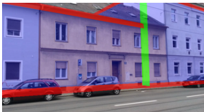
(j) Model reprojection using sensors estimation.
