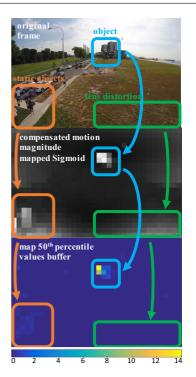
Figure 1: Example of spurious motion removal. (a) Original frame. (b) Magnitude of the compensated motion after mapping via a sigmoid function. (c) Difference from the learnt background indicating the presence of an incoming object.
