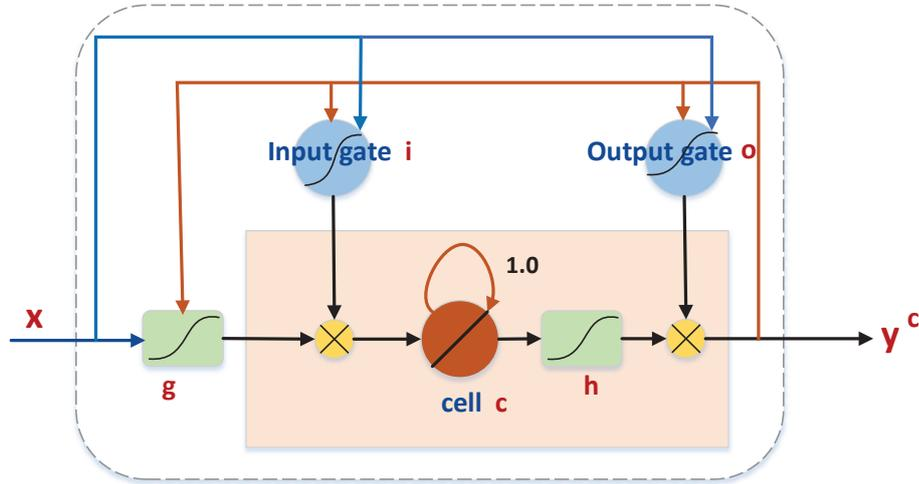
Figure 3: The structure of a LSTM cell neuron.
