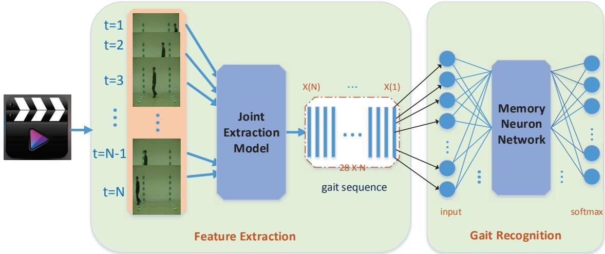
Figure 1: The Memory-based gait recognition framework. Obviously, the process is divided into two stages: feature extraction and gait recognition.  $N$  denotes the length of a gait sequence.
