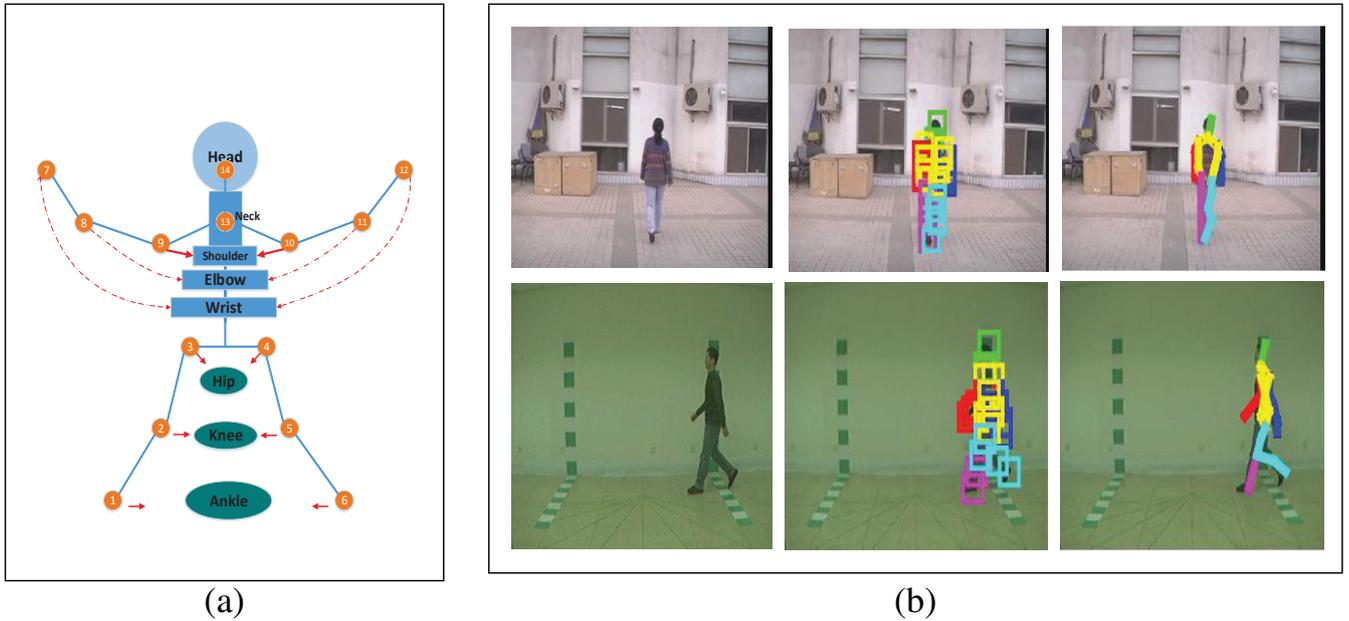
Figure 2: (a) A visualization of 14 body key points; (b) Two joint extraction samples. The left column is the input image. The middle and right column are part bounding boxes along with skeletons computed from the bounding boxes.
