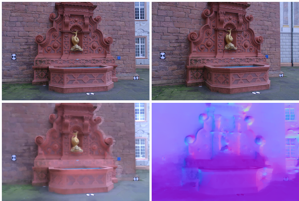
Figure 3: Real-world Fountain-P11 dataset [5]. Top row: Reference view (6), match view (7). Bottom row: Computed albedo, Computed illumination direction.
