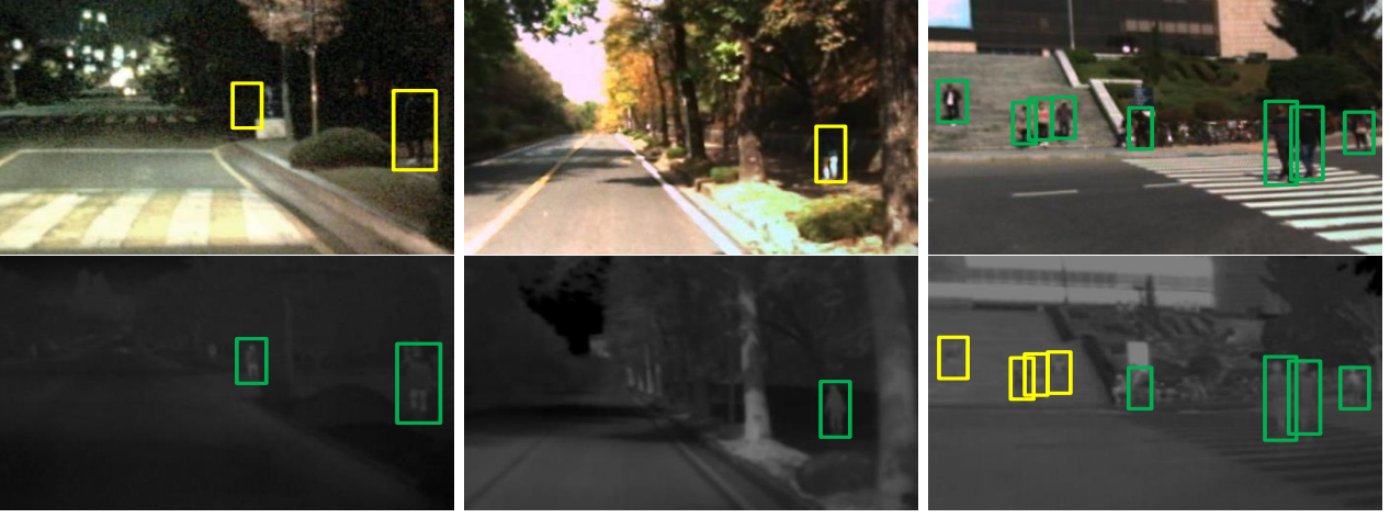
Figure 1: Left and middle: the thermal images capture human shapes even in bad lighting, while the corresponding color images are messed up. Right: with bright background, color image provides more distinctive visual features for the pedestrians (standing on stairs) against background objects; in such scenario, human silhouettes in the thermal image are ambiguous. Yellow bounding boxes indicate detection failures with one image channel.
