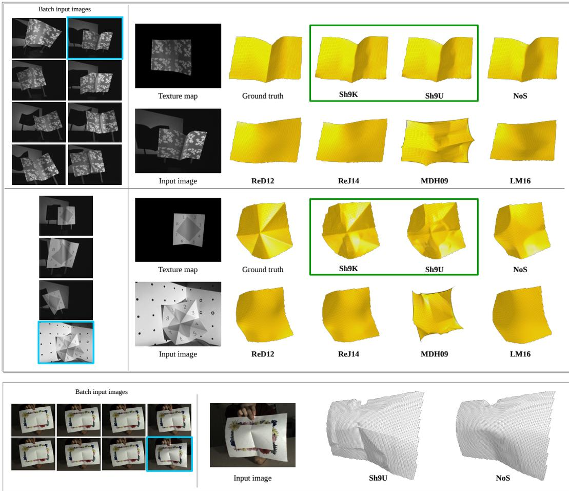
Figure 3: Renders of results. **Rows  $n^{\circ}1$  and  $n^{\circ}2$** : input image  $n^{\circ}5$  of the *floral plane* dataset. **Rows  $n^{\circ}3$  and  $n^{\circ}4$** : input image  $n^{\circ}4$  of the *paper fortune teller* dataset. **Rows  $n^{\circ}5$** : input image  $n^{\circ}8$  of the *floral video* dataset.
