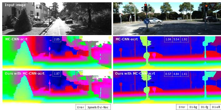
Figure 3: Example results of original MC-CNN-acrt and our fusion method with MC-CNN-acrt on KITTI 2012(left) and 2015(right).
