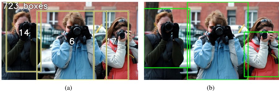
Figure 1: An example of human detection based on personness estimation: (a) The best matched windows generated by personness estimation: Total 723 candidate windows are generated, and 6th, 14th, and 17th windows are matched. (b) Human bounding boxes (BB) detected with the aid of candidate windows.
