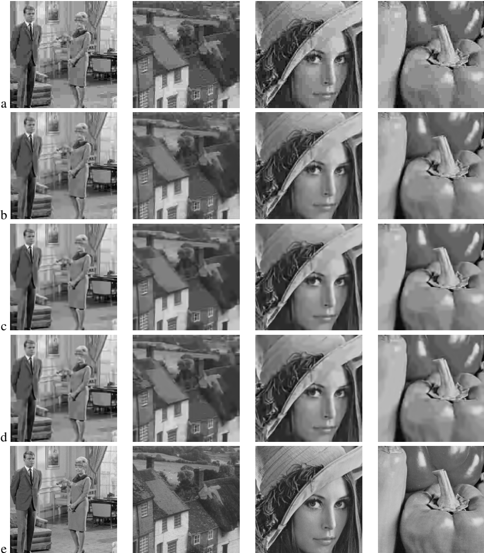
Figure 6: Comparison of the proposed method on (256 \times 256) -size sub-images: a. input JPEG images, b. SVR-based method [4], c. SADCT [4], d. the proposed method, and e. original un-encoded images.
