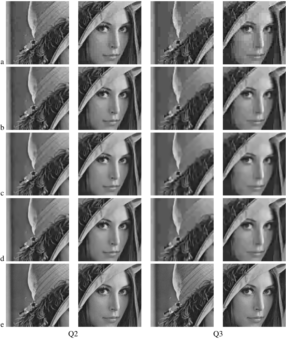
Figure 2: Example of artifact suppression for Lena image: a. input JPEG images, b. re-application of JPEG [10], c. SADCT [10], d. the proposed method, and e. original un-encoded images.
