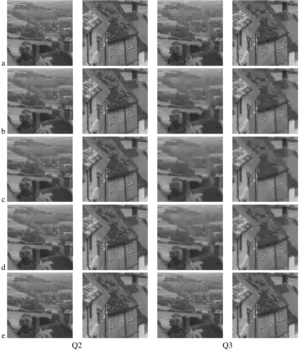
Figure 3: Example of artifact suppression for Goldhill image: a. input JPEG images, b. re-application of JPEG [10], c. SADCT [10], d. the proposed method, and e. original un-encoded images.
