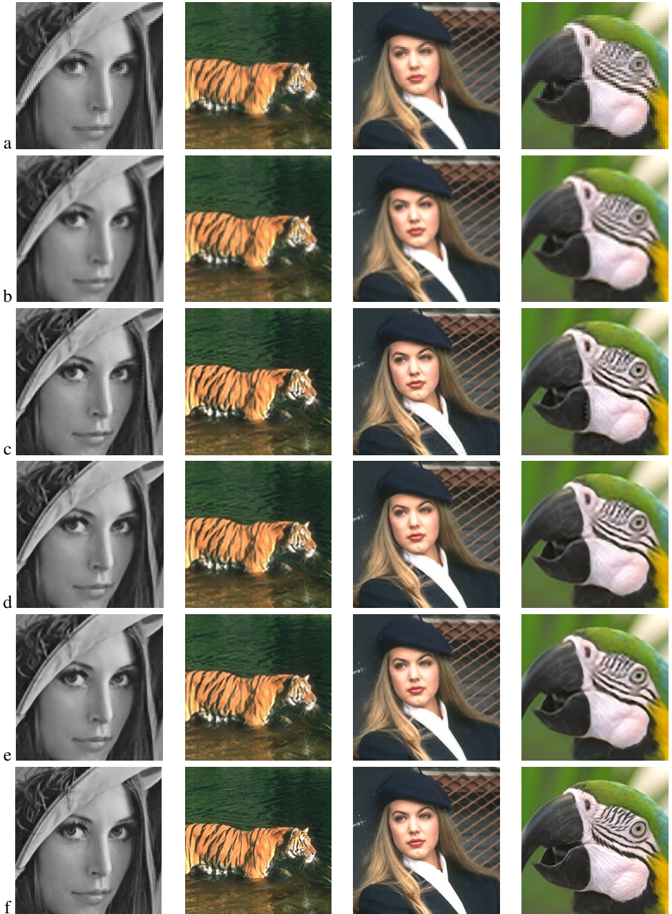
Figure 9: Examples of image super-resolution (magnification factor 3): a. nearest neighbor resampling, b. bicubic resampling, c. Yang et al. [14], d. Kim and Kwon [8], e. the proposed method, and f. ground truth high-resolution images.
