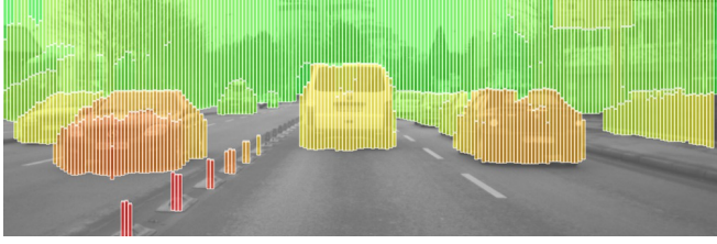
Figure 1: The multi-layer Stixel World result as output of the optimization. The captured scene is segmented into planar Stixel segments that correspond to either ground or object. The color represents the distance to the obstacle with red being close and green far away. Grey pixels belong to the ground surface.
