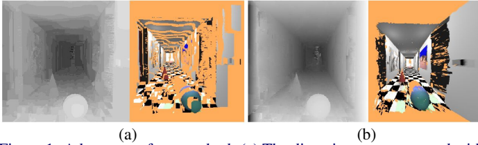
Figure 1: Advantage of our method. (a) The disparity map computed with fronto-parallel windows approximates slanted surfaces via many fronto-parallel ones. (b) Our slanted support windows correctly reconstruct the scene as a collection of slanted planar surfaces.
