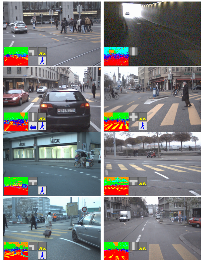
Figure 2: Example images. For each image, the bottom left shows the patch classification output, as well as the scene classification (road type, present objects). Figure is best viewed in color.
