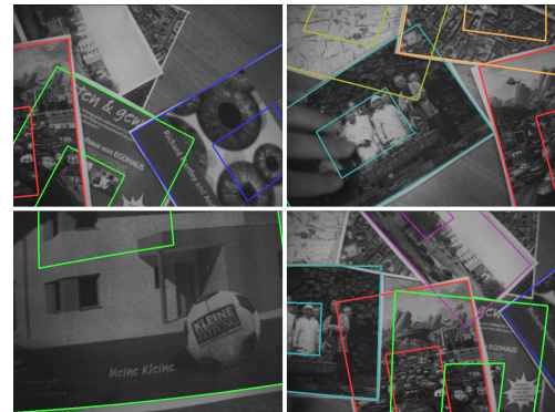
Figure 1: Four frames from a sequence demonstrating independent multiple object localisation. No frame-to-frame tracking is performed; the objects are localised in each frame. The mean total computation time per frame is 7.46ms using a single core of a 2.4GHz CPU.
