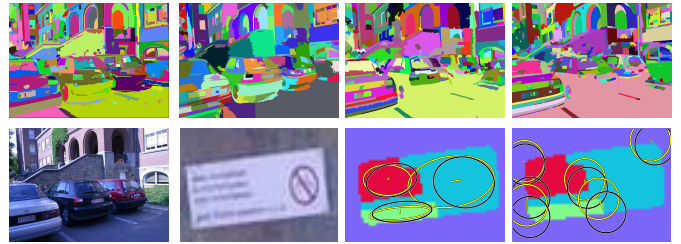
Figure 1: (Top) Segmentation maps of EGO, MS, NC, and WA on well-segmented set (left to right). (Bottom) Segment (third from left) and boundary (rightmost) based features (yellow) in the reference image together with their correspondences (black) projected from another image.
