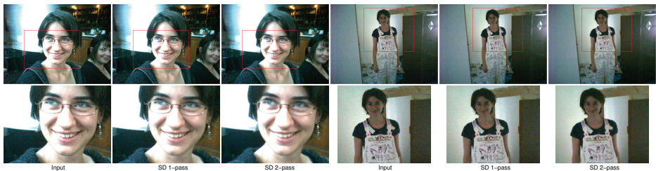
Figure 5: Noisy images from a cell-phone camera and detail crops. These photographs show that for heavily corrupted images, the two pass algorithm achieves excellent denoising results.
