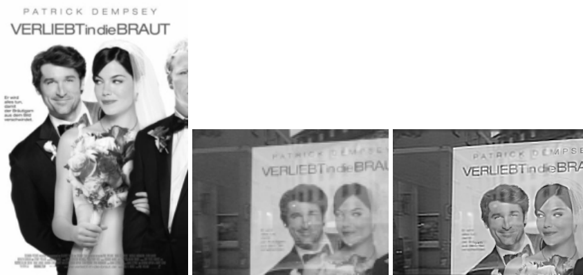
Figure 8. Left: high-resolution still image, Middle: low-resolution video frame, Right: MAP superresolution with Huber-prior and high-resolution prior.
