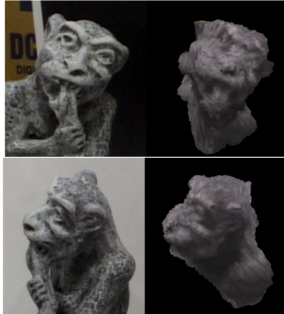
Figure 7: Two views of the gargoyle model with corresponding reconstruction. We rendered the reconstructed model by associating to each vertex the average projected color of the corresponding voxel.
