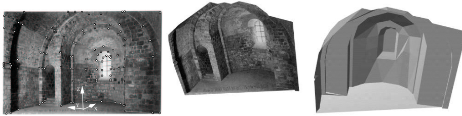
Figure 4: Left: Indoor scene with 114 identified points. Middle and Right: Reconstruction, shown with and without texture, obtained from these points and 39 known planes.
