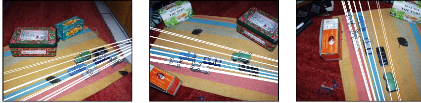
Figure 5: Motion line pencils estimated using two-view projective bundle adjustment between the first and the second views and constrained estimation of a 5-dof C-tensor between the second and third views. Note that the motion lines pencils are perfectly aligned in the second image.
