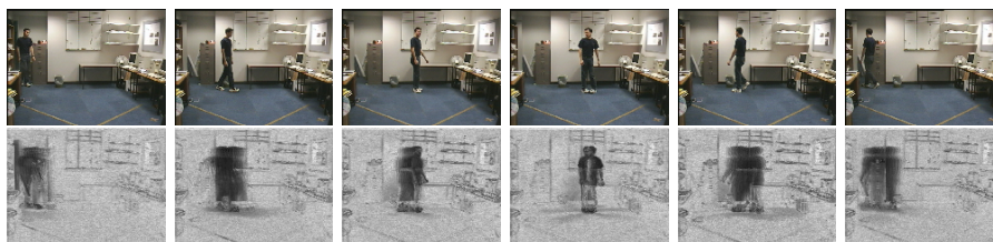
Figure 1: Rows from top to bottom: (a) Selected frames from a left-right-left walking sequence. (b) Pixel-energy data is encoded in grey-level using a log-scale to show small scale structures. (Black indicates high response). Reflective edges can be seen with small responses.
