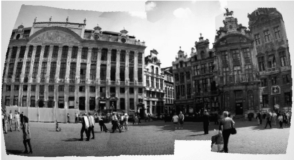
Figure 3: The five images from the Market Square sequence stitched together. The visible image boundaries are not registration errors, but brightness variations between and within images, which we do not currently model. Indeed the centre of each image is significantly brighter than the periphery.
