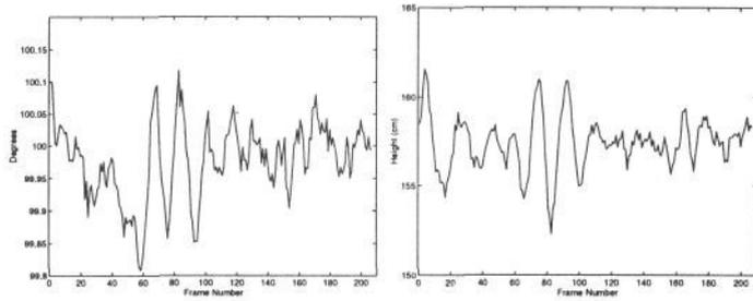
Figure 10: Camera inclination angle and camera height estimated from ground plane disparities for a freeway driving sequence.
