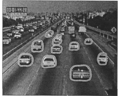
Figure 5: Vehicle occlusion can be predicted from the depth ordering of vehicles. Information in the occluded region must be extrapolated for the more distant vehicle. The figure on the right contains a partially occluded vehicle.
