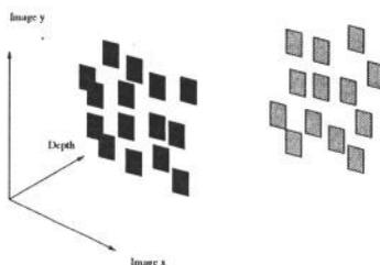
Figure 8: Connected components in image/depth space consist of those pixels which are nearest neighbors in image coordinates as well as having depth differences less than depth uncertainty.
