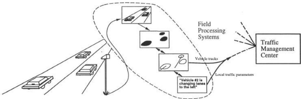
Figure 1: Our system concept for video traffic surveillance.
