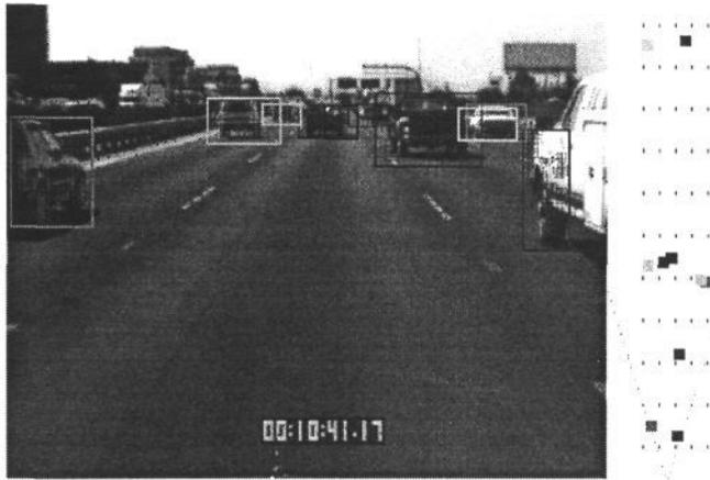
Figure 9: Objects identified as being in the same lanes of traffic as the test vehicle. On the right side of the image is a bird's-eye-view from above the road surface showing the relative position of the tracked objects with respect to the test vehicle.
