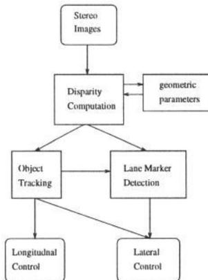
Figure 6: Block diagram of the stereo-based vehicle control system. Arrows indicate flow of information.
