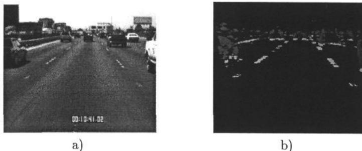
Figure 7: a) left image and b) light indicates objects were detected to be on the road surface, dark indicates objects are above the road surface, black indicates regions where the disparity could not be accurately recovered.
