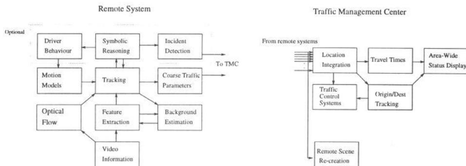
Figure 4: Block diagram of the complete traffic surveillance system.
