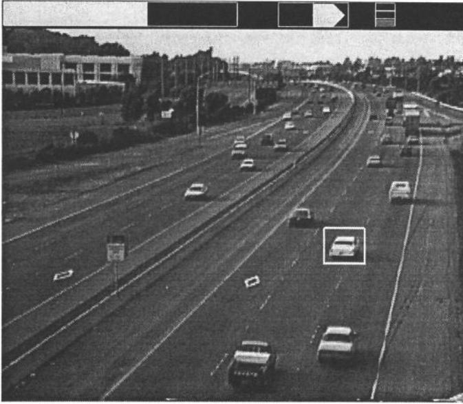
Figure 2: Highway scene (I-580 in Richmond, CA) showing tracking information for the car outlined. The bar at the top shows the vehicle's speed. The arrow at top is the lane change indicator. The indicator at top right is green to show that the vehicle is operating normally (i.e., not stalled).
